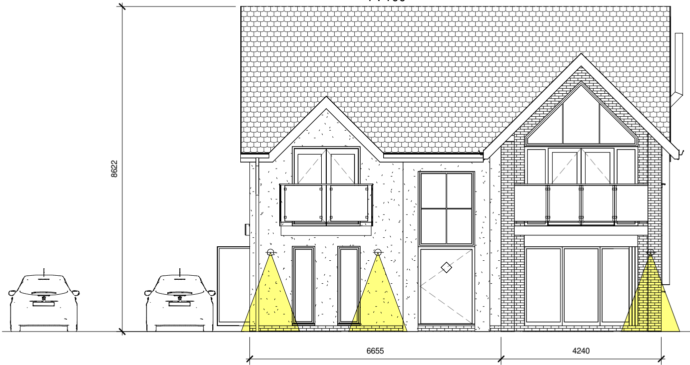
2 Front Elevation Lighting 1 : 100
