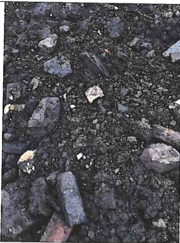
Plate 2: Stockpile 1A of black-grey made ground containing fine gravel to boulder-sized fragments of concrete, brick, wood, pipes, and linoleum.
