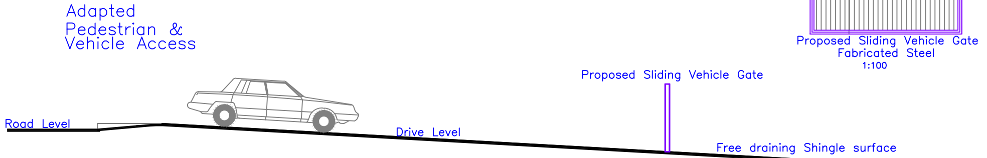
Proposed Section Drive Access to Car Park 1:100
