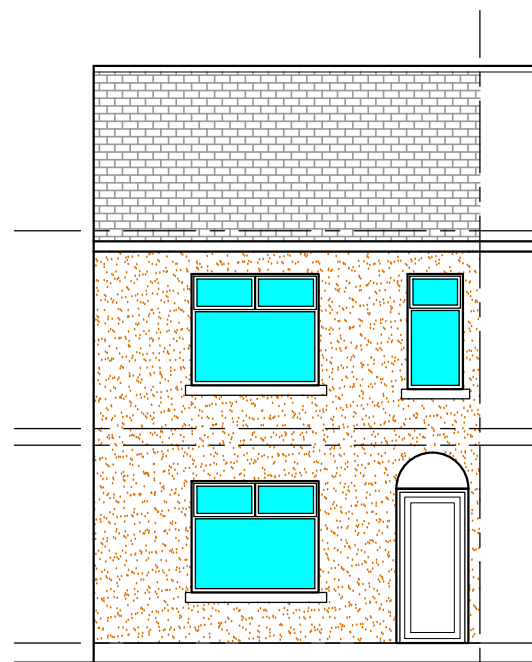
FRONT ELEVATION AS EXISTING 1:100
