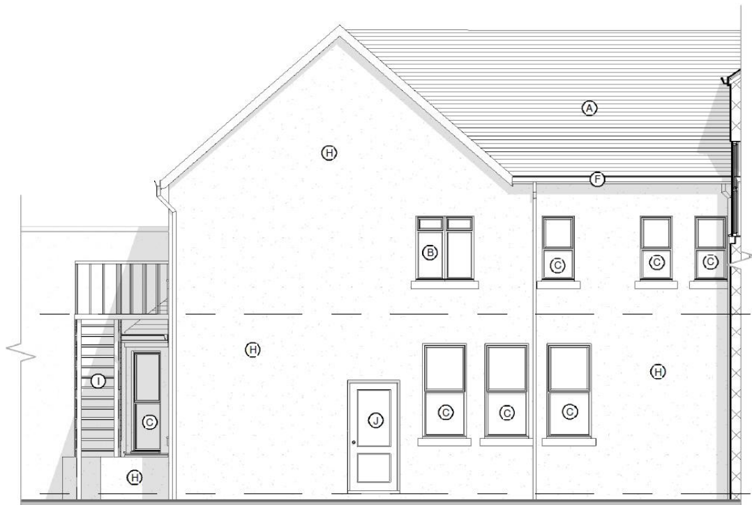
Figure 7. Existing north elevation.
