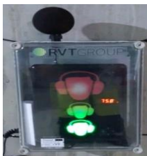
Fig.3.1 – Noise Monitoring Stations to be used
