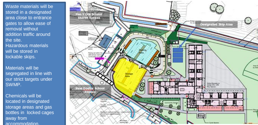
Fig.3.4 – Recycling area – waste segregation – extract from main Construction Site Layout
