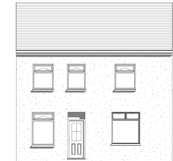
3 Existing Front Elevation 1 : 100
