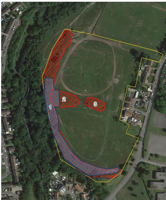
Figure 7 – Area for deposition of topsoil containing Japanese knotweed rhizomes
