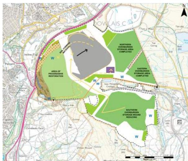
As identified above, the site has been progressively worked from a southwest to northeast direction; with the current working face located on the eastern edge of the void and backfill of material taking place on the western edge of the void. This working has been split across 25 'cuts' which provides a clear working practice across the site. The final cut at the site was undertaken in two stages, with cut 25B ongoing at present.
