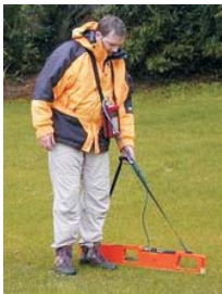
EM-38 Single frequency Exploration depth ~1.5m
