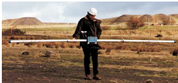
EM-31 Single frequency Exploration depth ~3 to 5m
