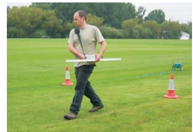
GEM-2 Multi-frequency Exploration depth up to 10m
