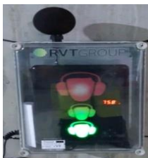
Fig.3.1 – Noise Monitoring Stations to be used
