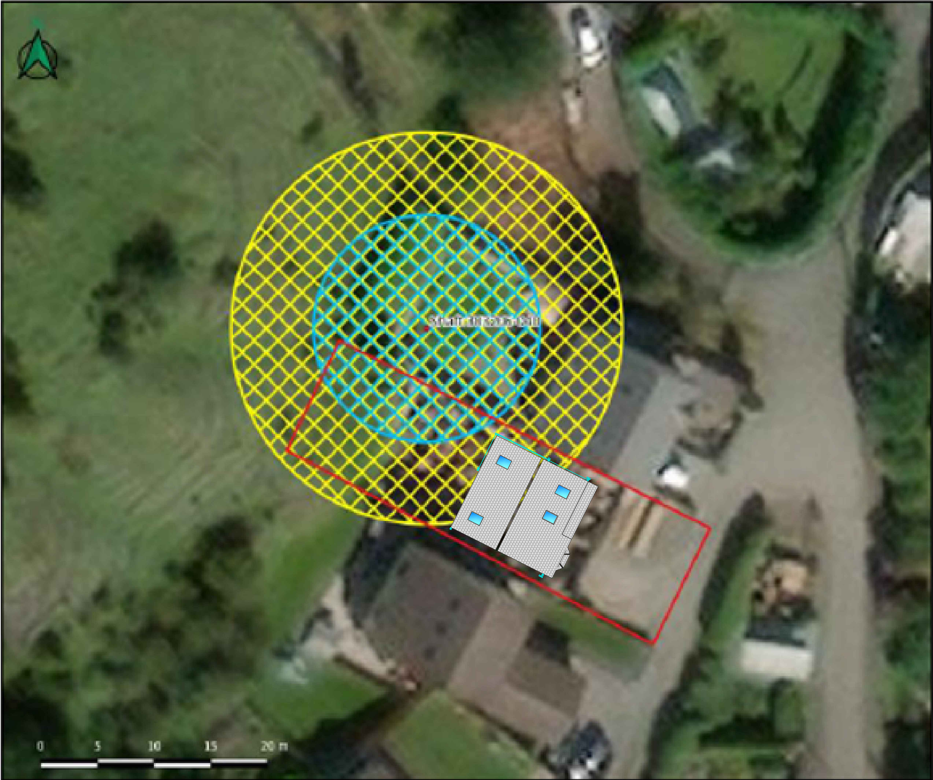
Figure 3.1: Shaft location, departure zone and exclusion zone
