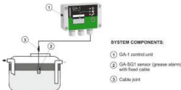
Figure 1. Grease separator supervision with GA-1 alarm device
