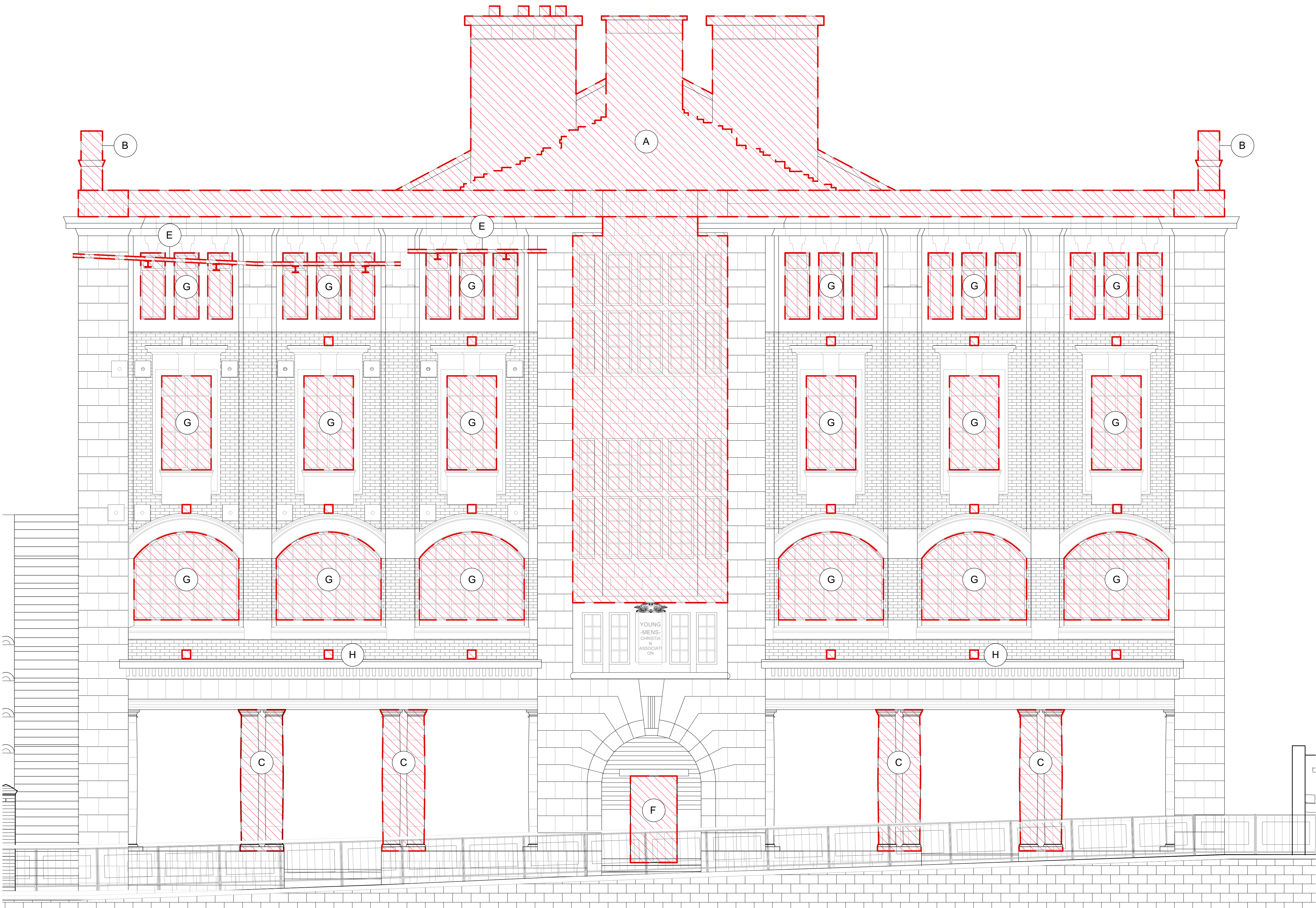
1 South Demolition Elevation Scale: 1:50
