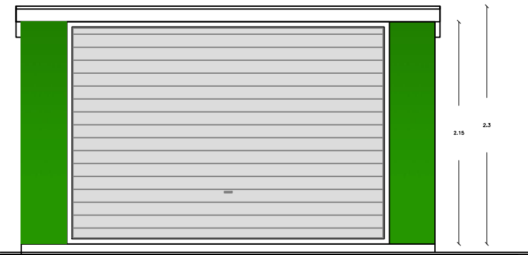
Proposed New Dugout Front Elevation 1:50
