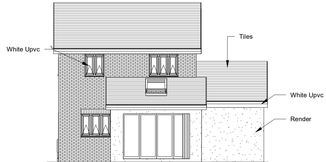
2 Existing Rear Elevation 1 : 100
