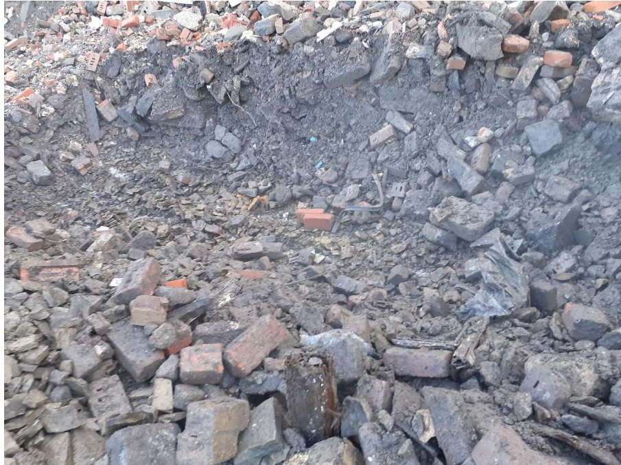
Plate 29: Excavation into Stockpile 8D showing coarse gravel to cobble sized fragments of demolition material.
