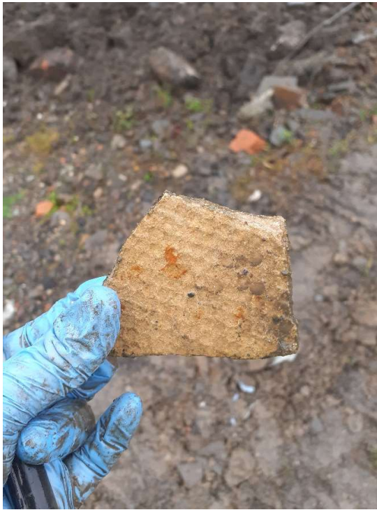
Plate 21: Fragment of asbestos cement on surface of Stockpile 6C.
