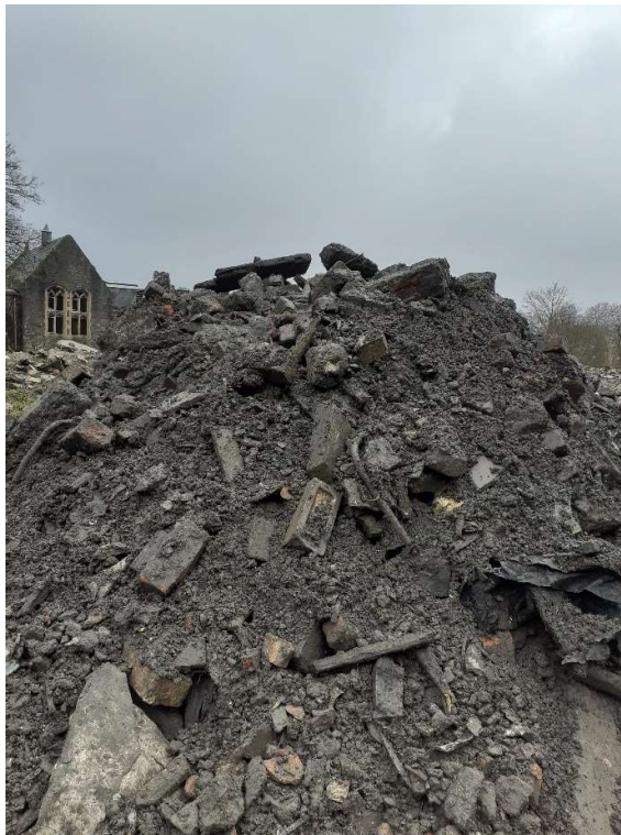
Plate 16: Black-grey gravelly bouldery clay material of Stockpile 6A.
