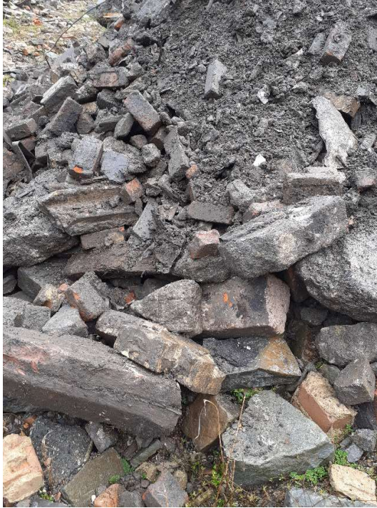
Plate 17: Coarse gravel to boulder-sized concrete, brick, wood, tile, and wire material in Stockpile 6A.
