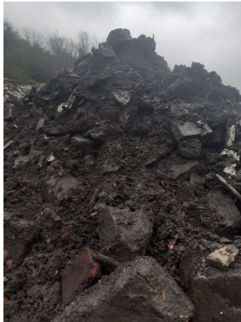
Plate 27: Clayey ash fill with coarse gravel to boulder-sized fragments of concrete, brick, pipes, wood, tile plastic strips and metal of Stockpile 7C.
