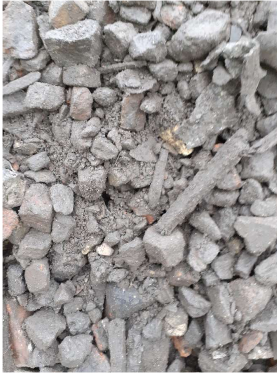
Plate 15: Fragments of concrete, brick, wood, and plastic tile in Stockpile 5A.
