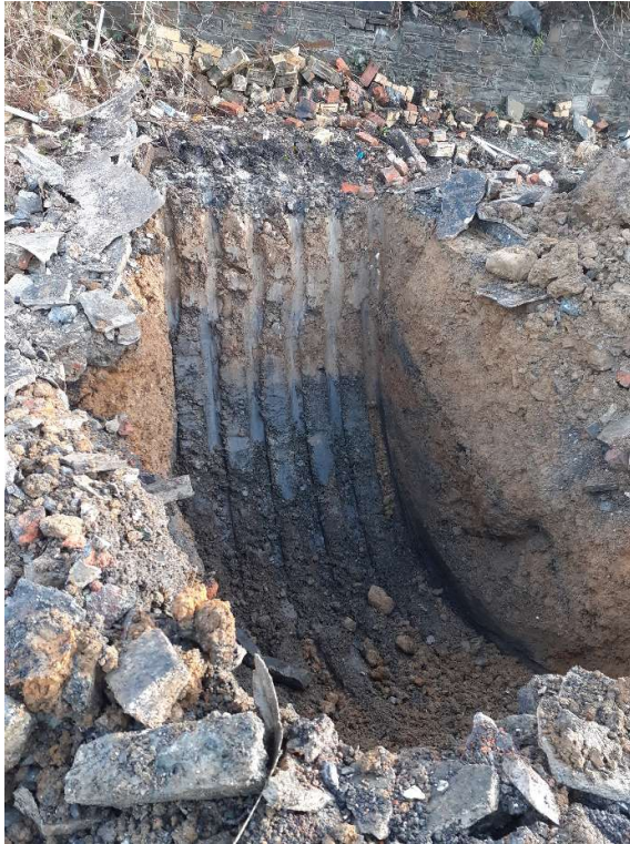
Plate 31: Excavation into Stockpile 9B showing natural clay underlying made ground.
