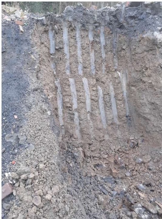
Plate 28: Excavation into bank behind Stockpile 8C showing natural clay underlying the made ground surface.
