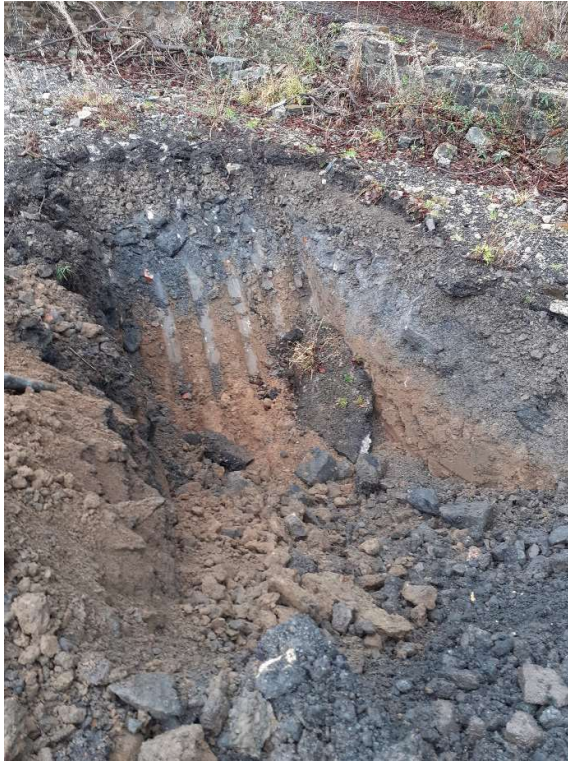
Plate 25: Tarmac and coarse roadstone over natural brown clay of Stockpile 7A.
