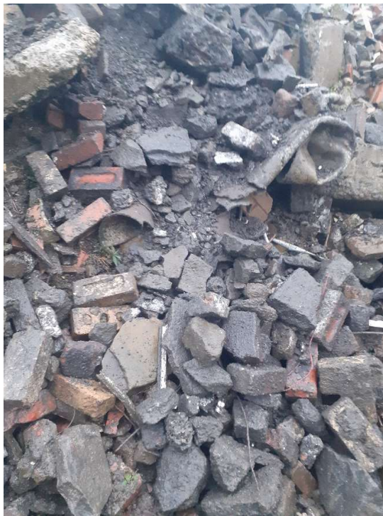
Plate 24: Cobble to boulder-sized fragments of concrete, brick, pipe, fabric, and concrete slabs of Stockpile 6D.
