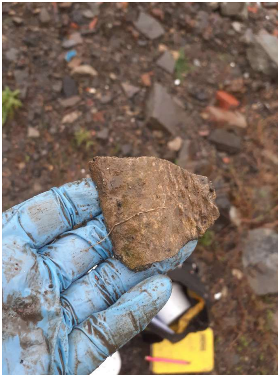
Plate 22: Fragment of asbestos cement on surface of Stockpile 6C.
