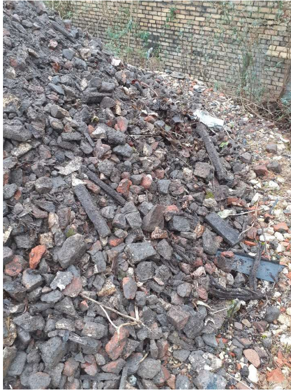
Plate 9: Made ground gravel encountered in Stockpile 2A, showing coarse to cobble-sized fragments of brick, concrete, plastic tile, and wood.
