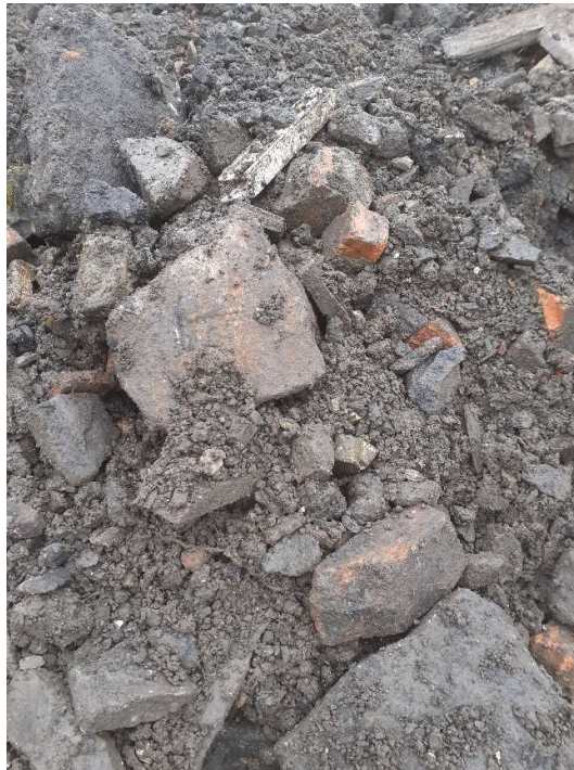
Plate 3: Stockpile 1C of black-grey made ground containing fine gravel to boulder-sized fragments of concrete, brick, wood, plastic strips, and slate.
