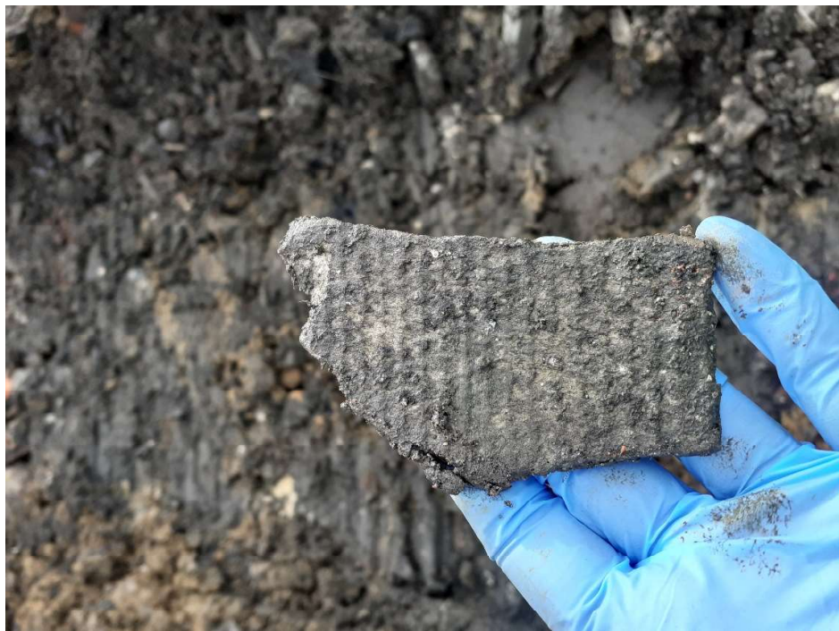
Plate 34: Fragment of asbestos cement on surface of Stockpile 9C.
