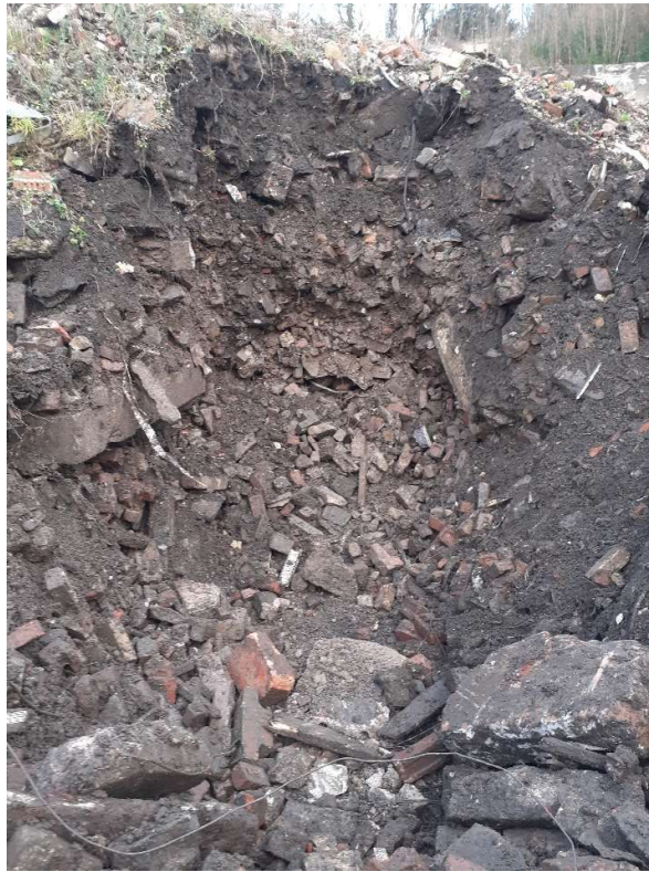
Plate 37: Excavation into Stockpile 10C, showing coarse gravel to boulder sized fragments of brick, wire, rebar, pipe, concrete, concrete block, and white tile.
