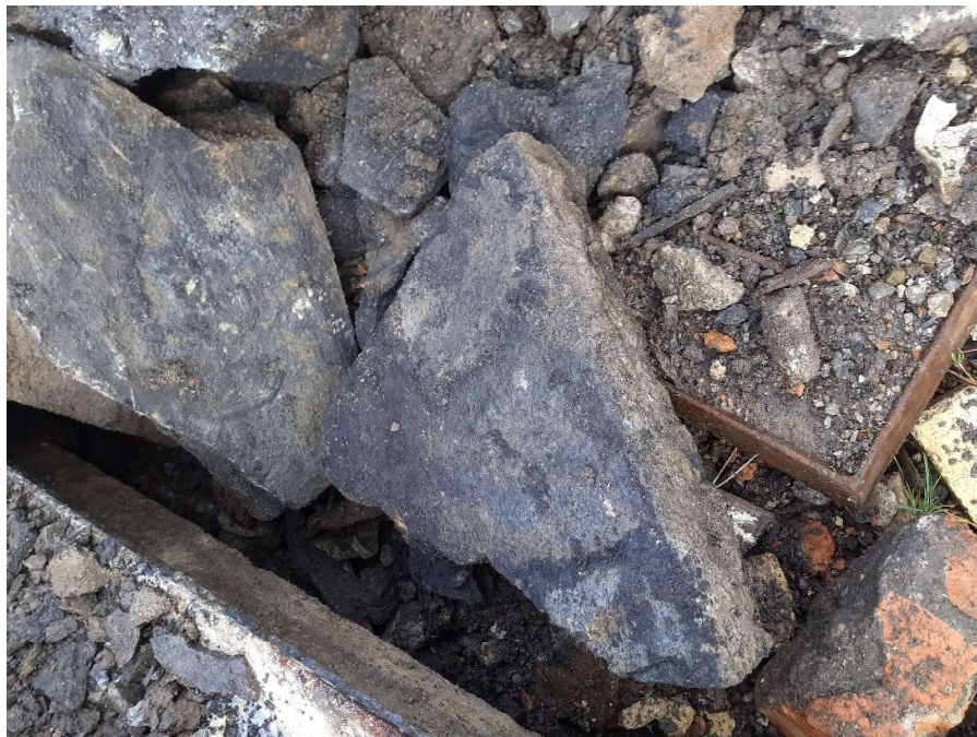
Plate 32: Fragments of concrete with bituminous coating on base of Stockpile 9C.
