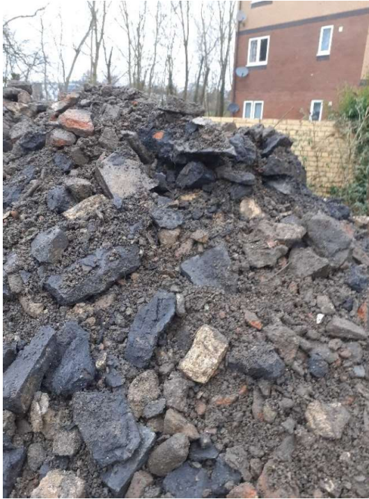
Plate 11: Fragments of black tarmac encountered at base of Stockpile 2A.
