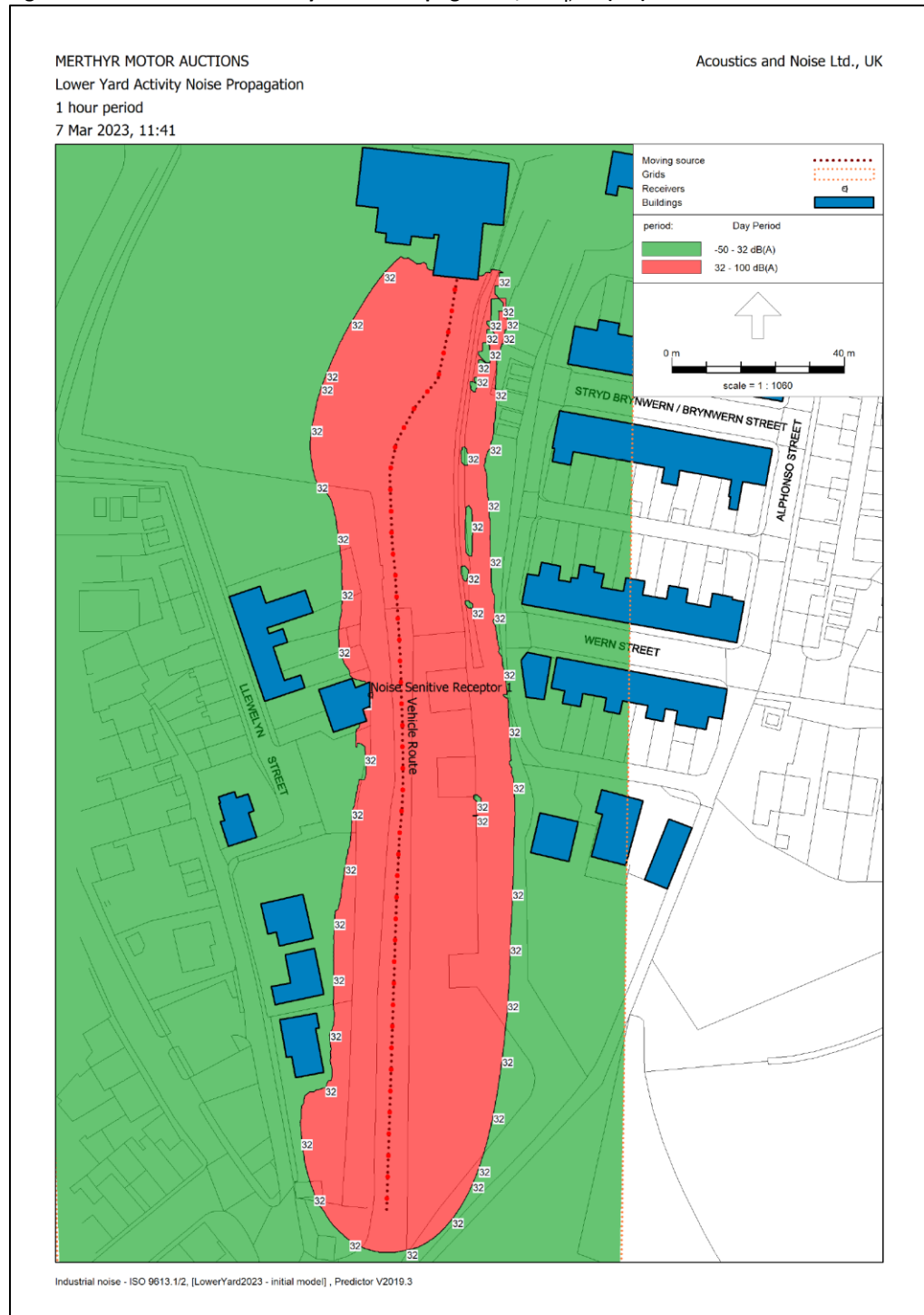
Figure 4 – Lower Yard Activity Noise Propagation, L_{Aeq,1hr} (dB)
