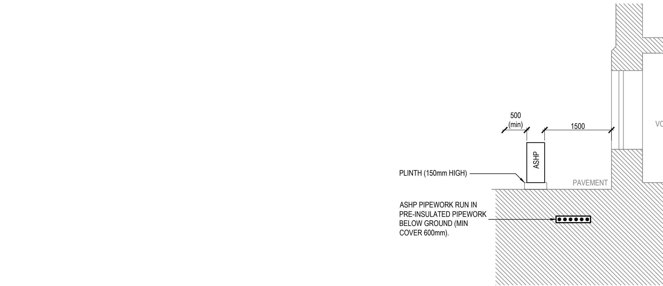
SECTION C-C (PART ONLY - LGF ASHP EXTERNAL) SCALE 1:50
