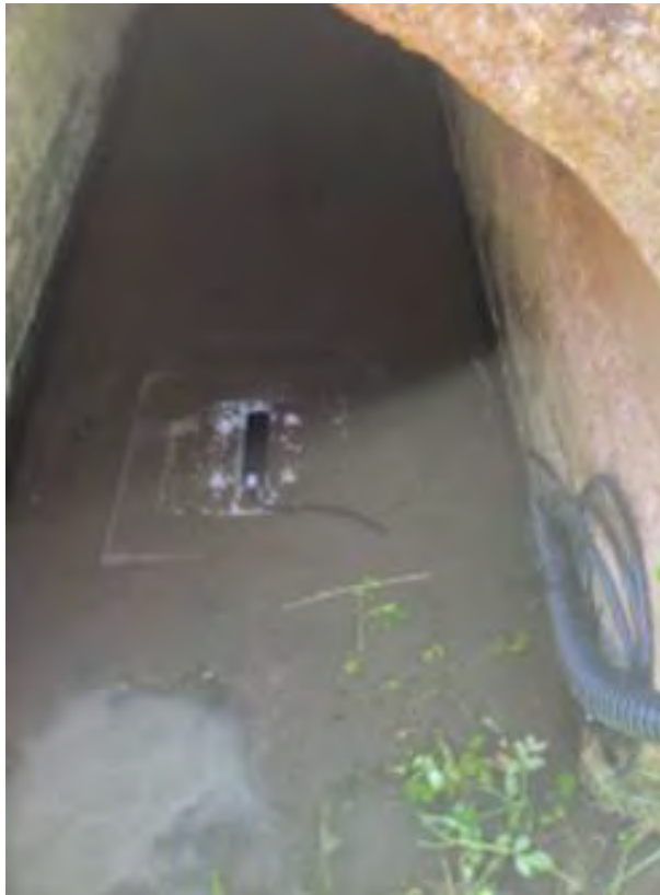
Figure 5: ISCO Area-Velocity AV350 doppler sensor
