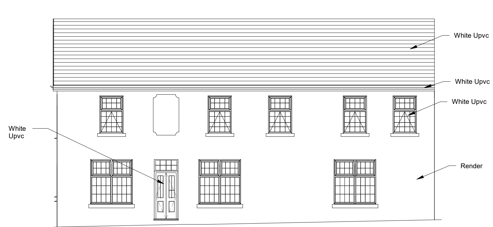
Existing Front Elevation
