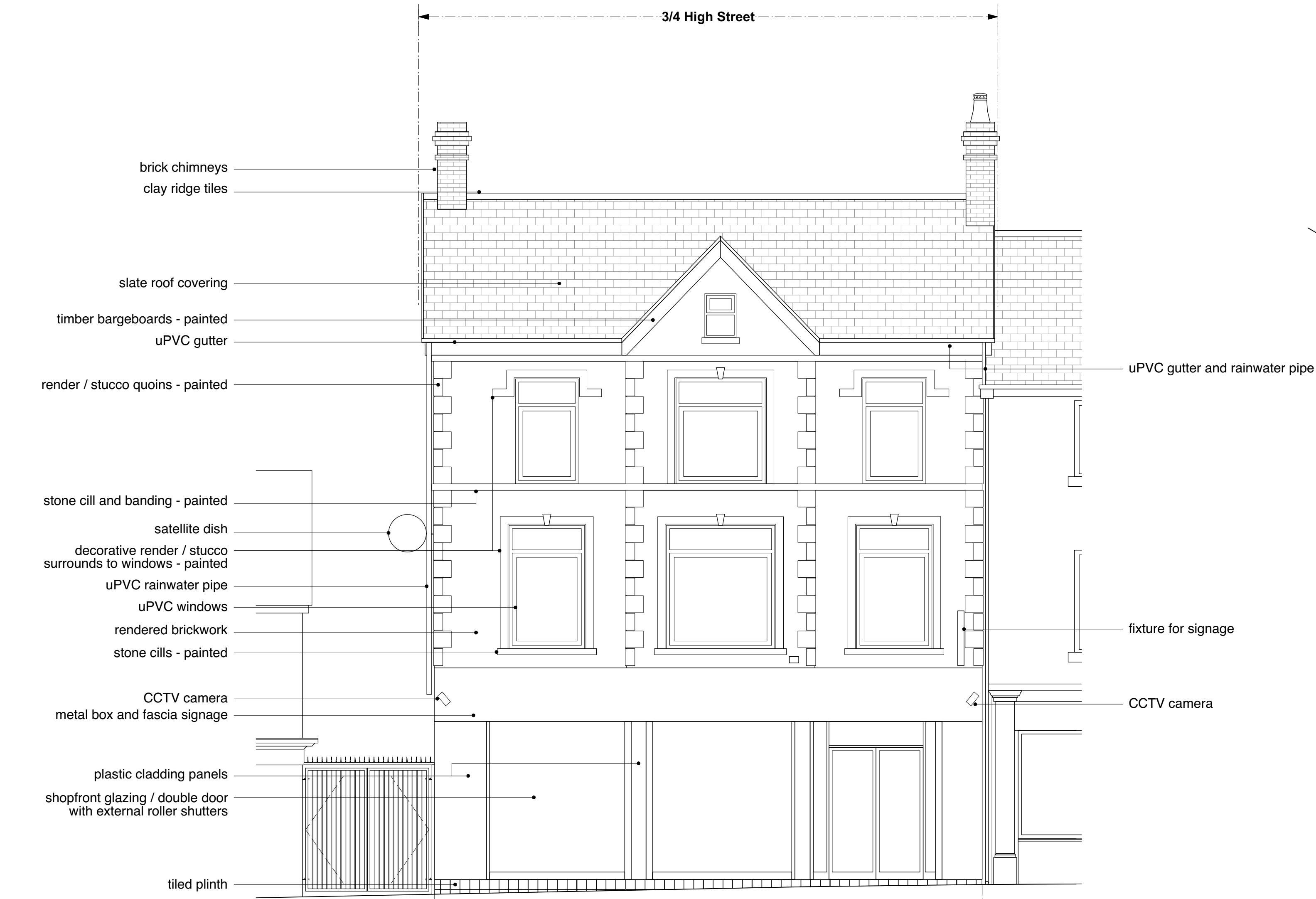
01 existing: front elevation (not surveyed)
