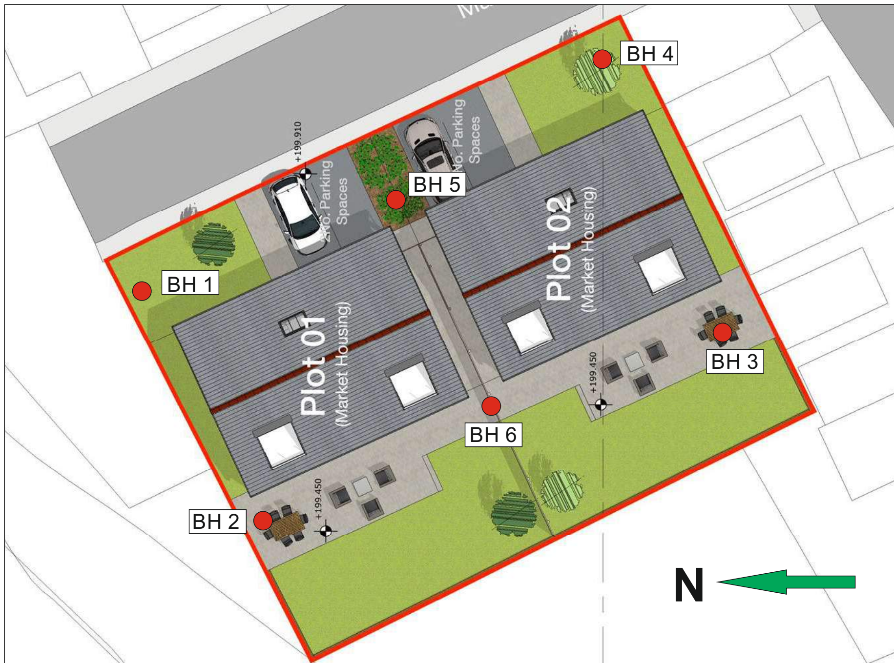
FIGURE 7 BOREHOLE POSITIONS AS DRILLED AT MARDY ST.
