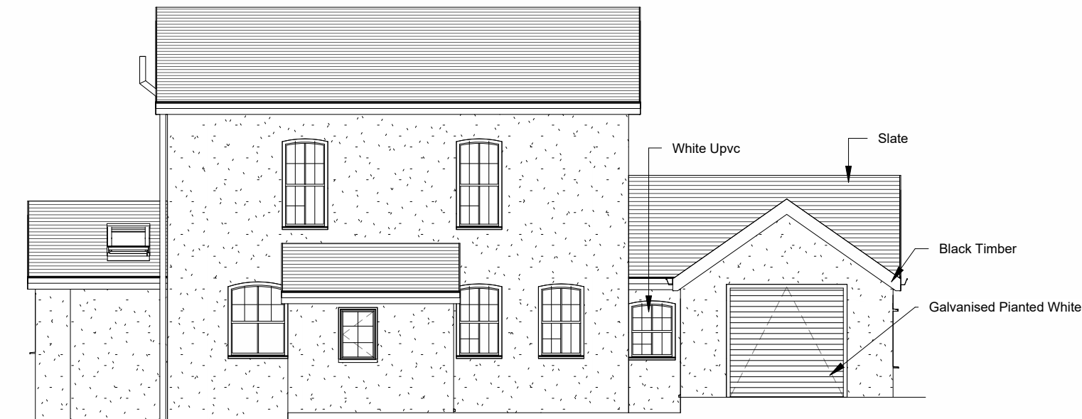
1 Existing Front Elevation 1 : 100
