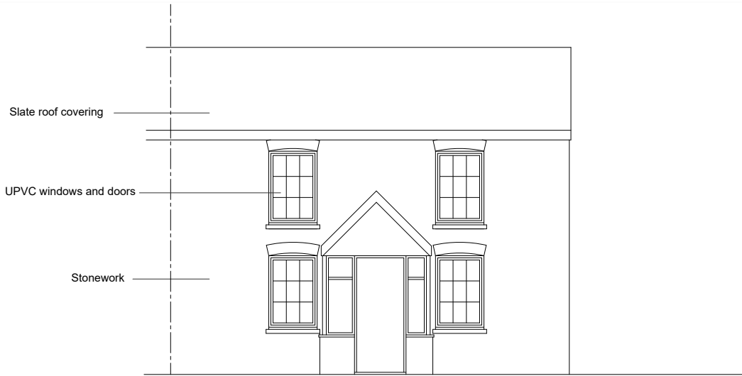
EXISTING FRONT ELEVATION
