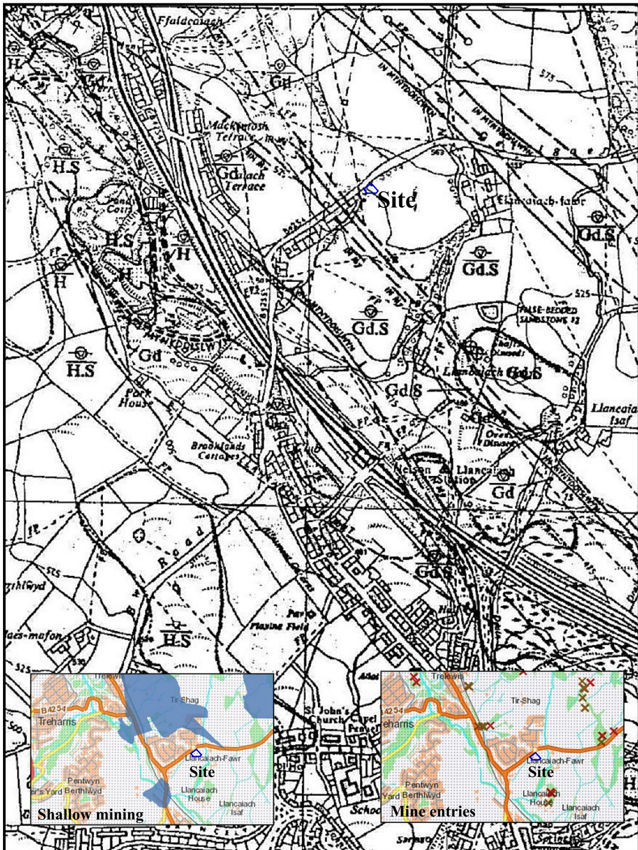
Fig. 2 Proposed development off Gelligaer Road, Trelewis; Geological plan with mining details (inset)
