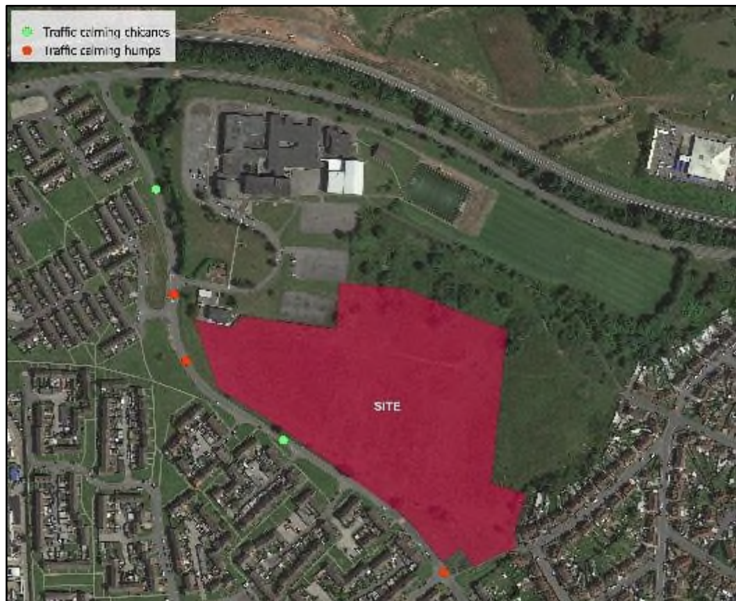
Figure 2.3 Existing traffic calming on Goitre Lane
