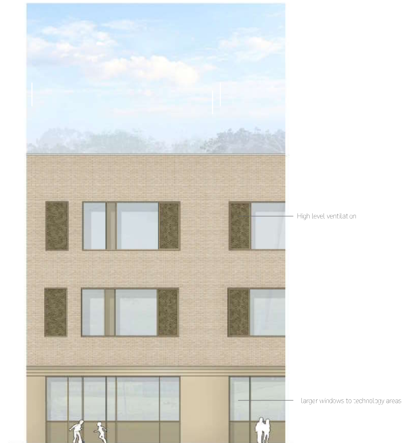
Detailed elevation to secondary classroom wing
