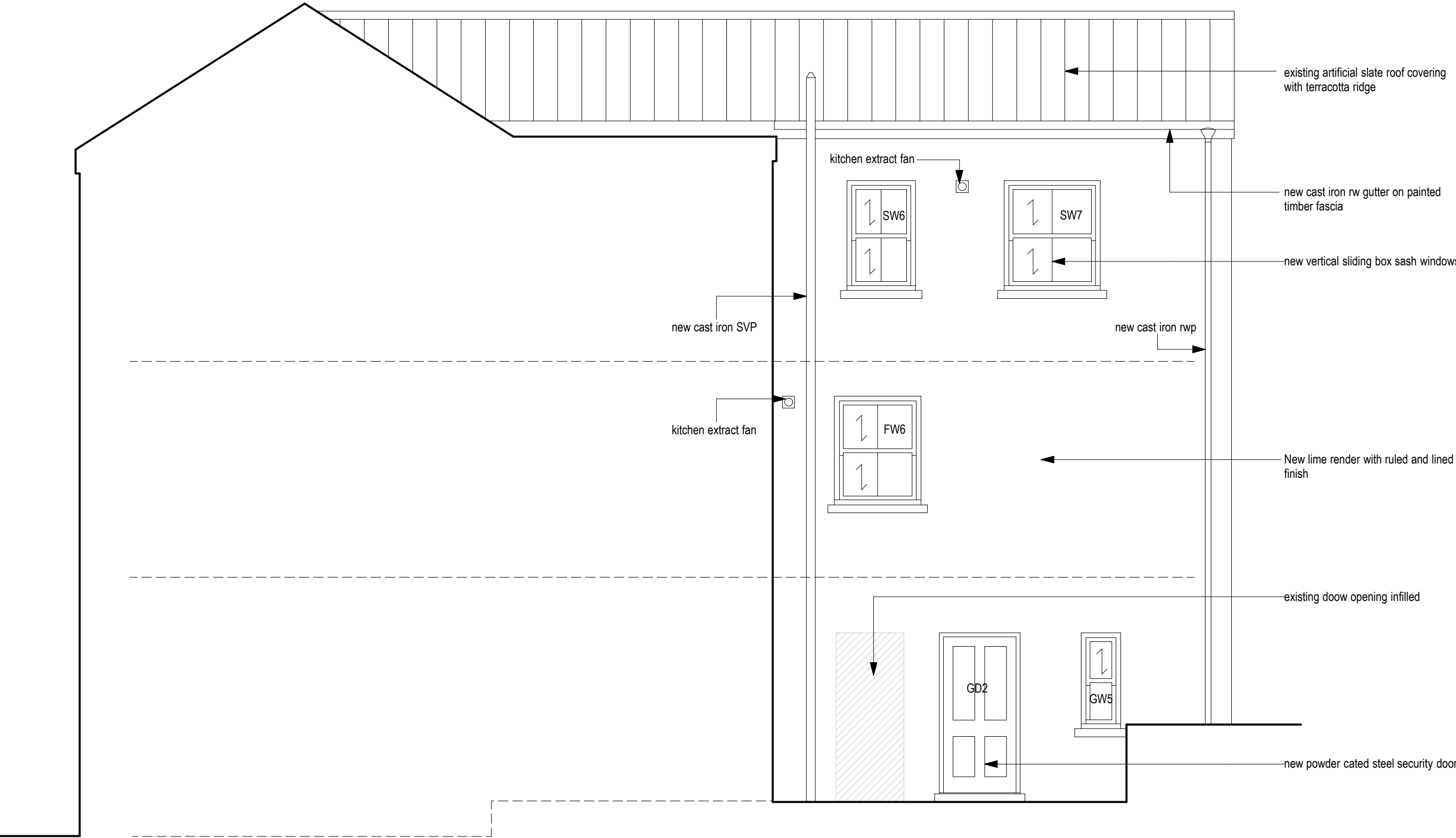
ELEVATION TO SIDE OF REAR EXTENSION
