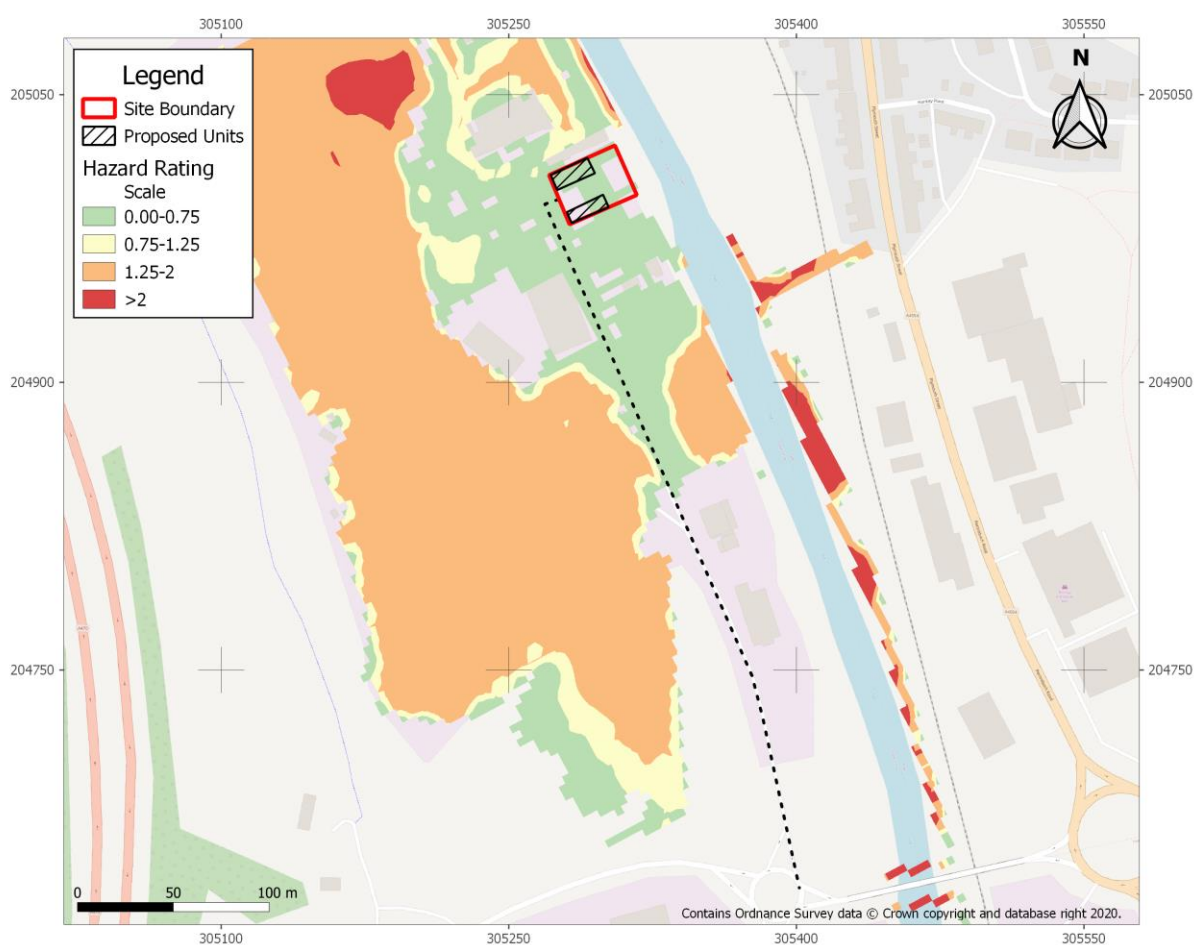
Figure 4-4 - Access/Egress (1 in 1000yr event hazard map)
