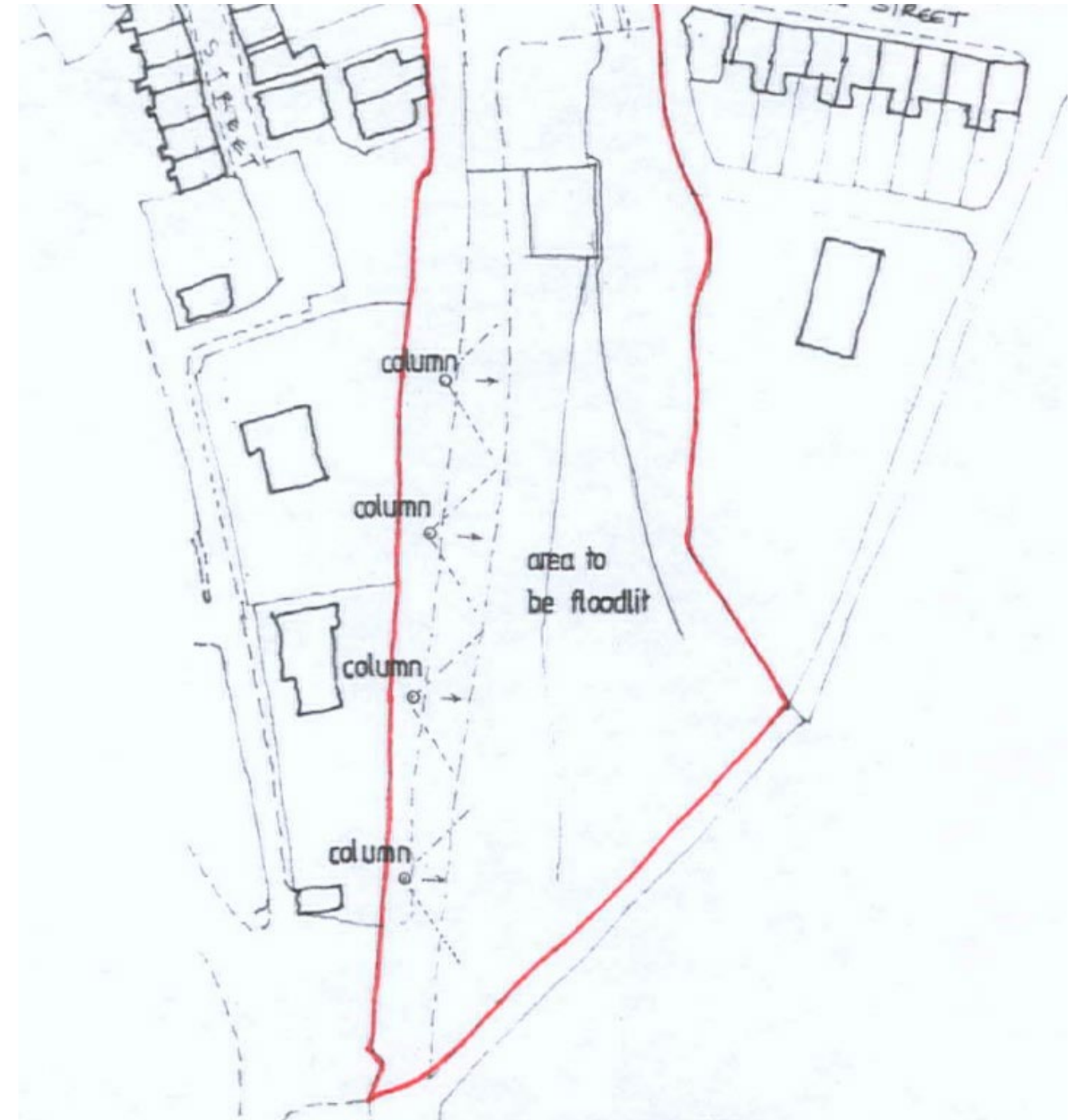
Existing lighting installation layout
