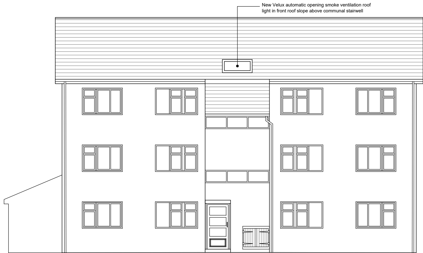
FRONT ELEVATION AS PROPOSED @ 1:100
