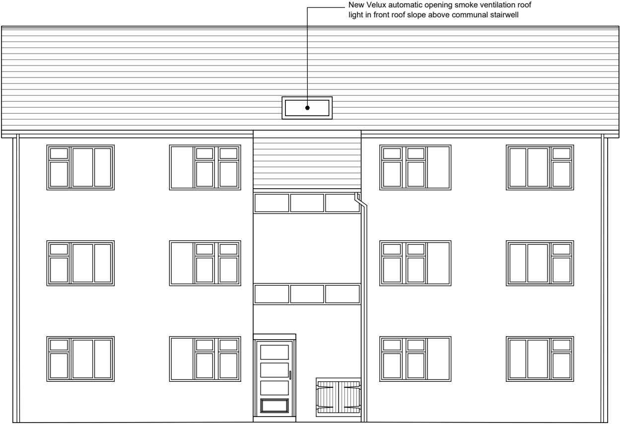
FRONT ELEVATION AS PROPOSED @ 1:100
