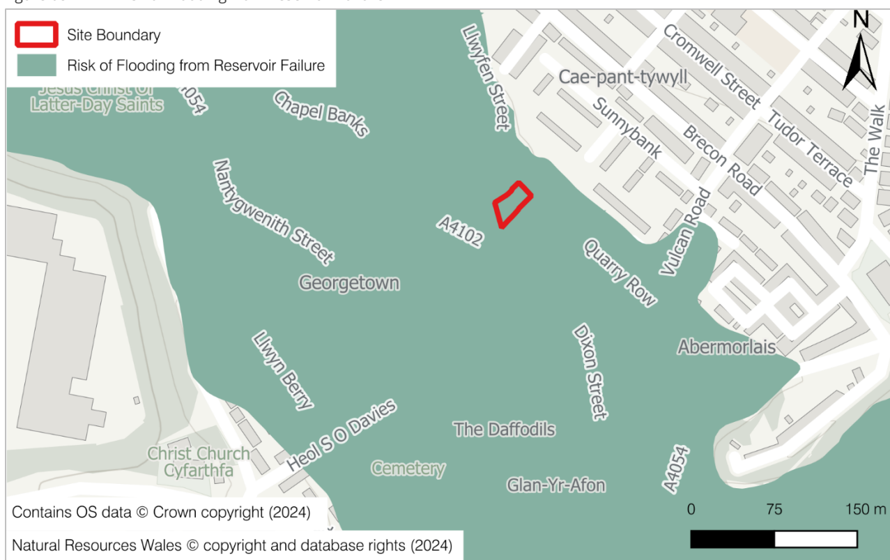
Figure 08 - NRW Risk of Flooding from Reservoir Failure
