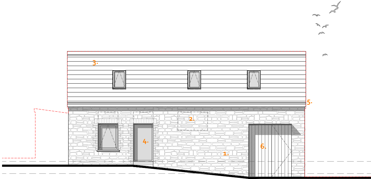
Front Elevation (West)
