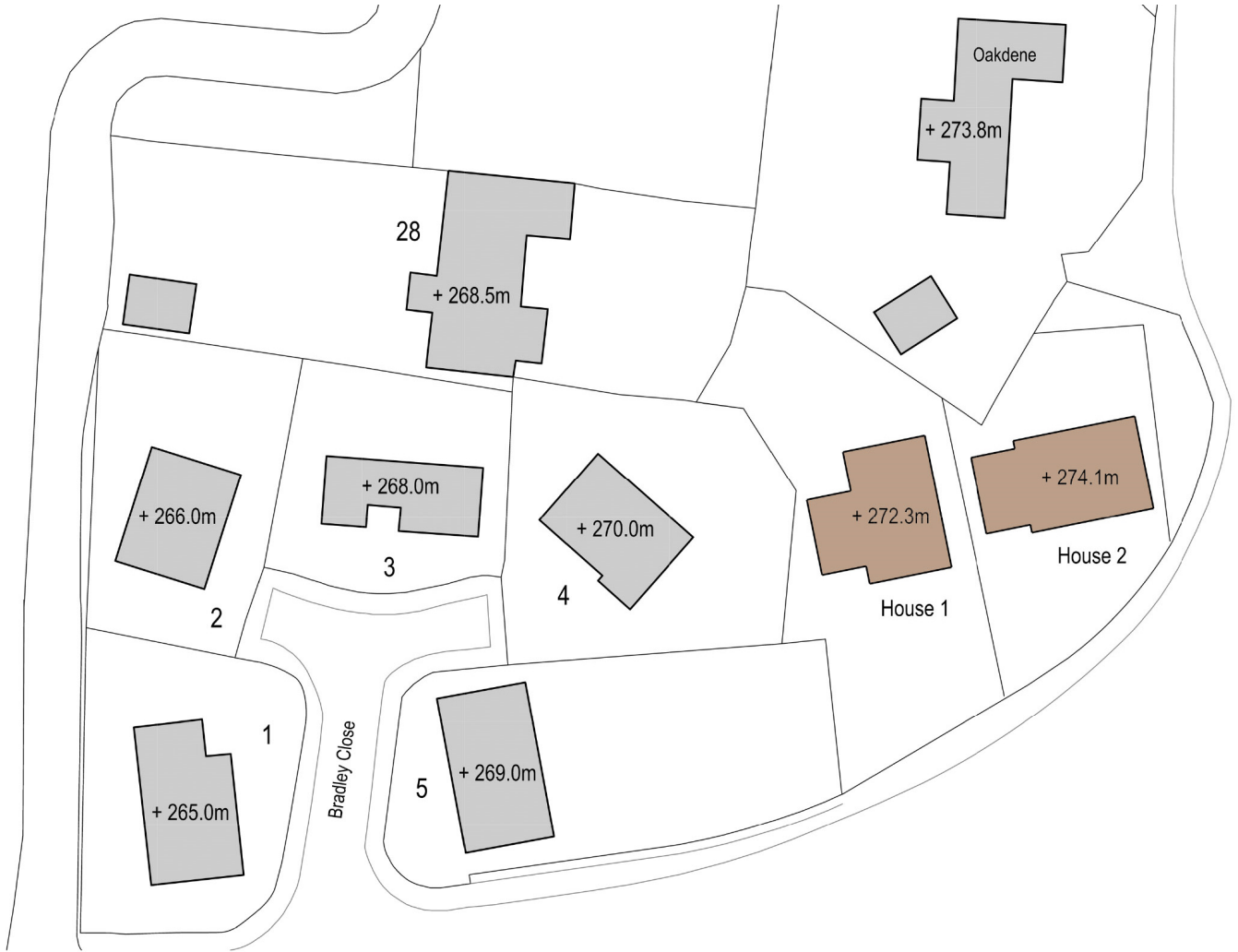
Fig 6 Ground floor levels of existing and proposed houses.
