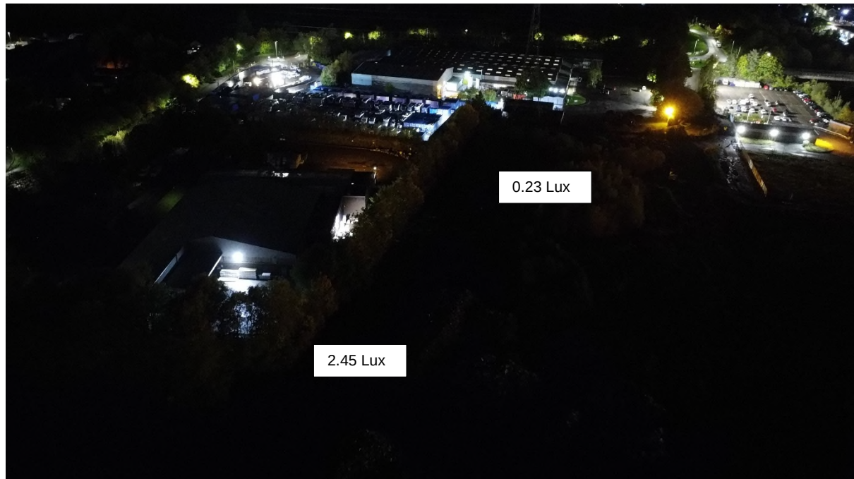
Plate 11 Showing west boundary and north boundary light spill
