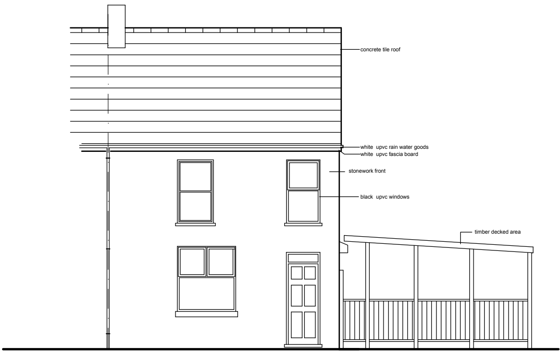
EXISTING FRONT ELEVATION
