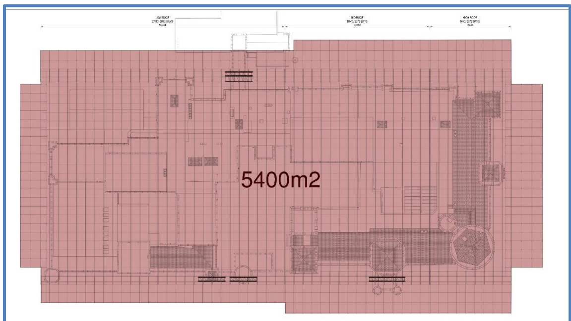
Figure 4 Approximate temporary scaffold roof area
