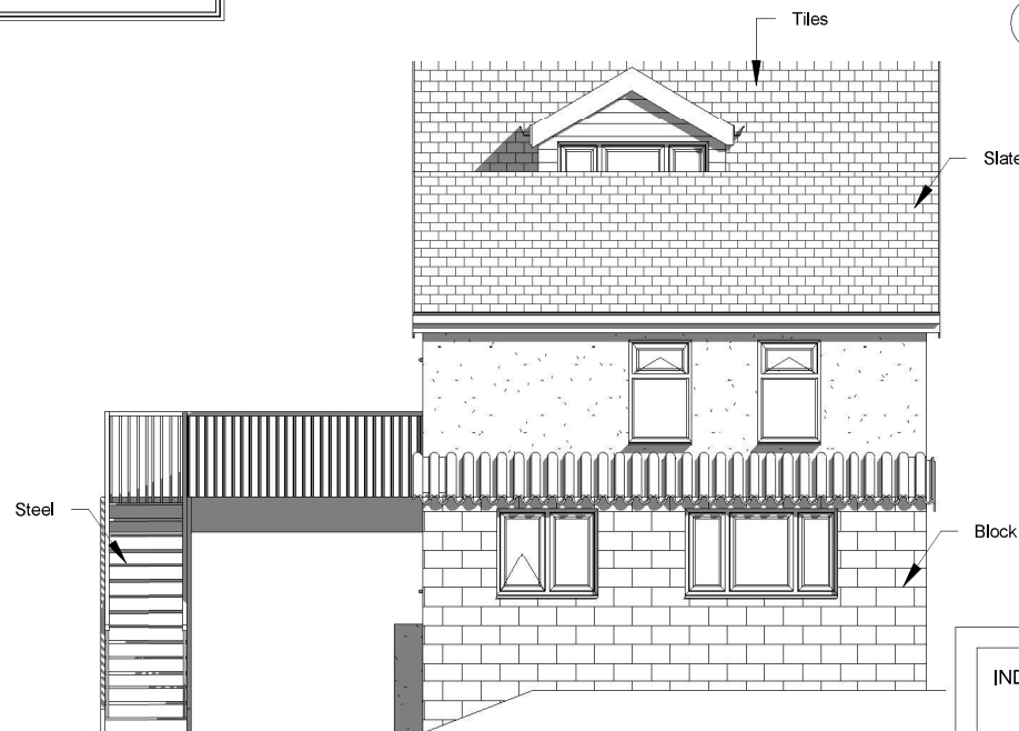
6 Existing Rear Elevation 1 : 100
