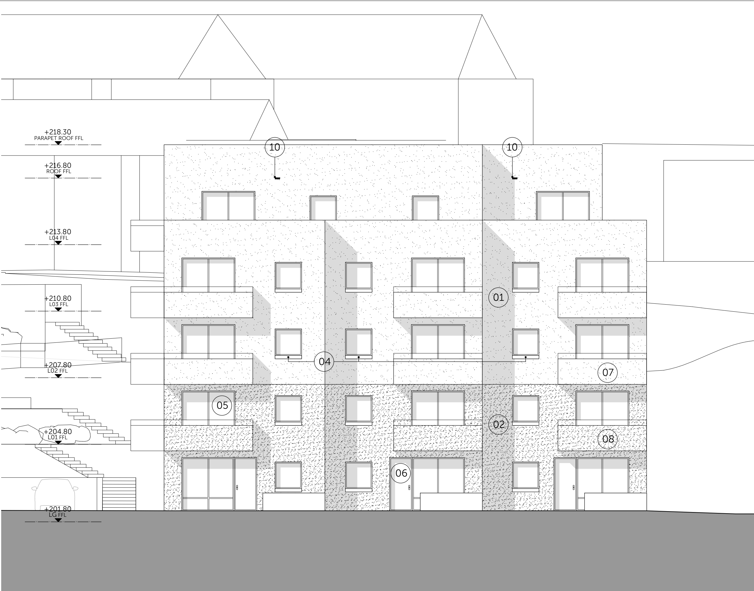
2. SOUTH ELEVATION BLOCK B - BB
