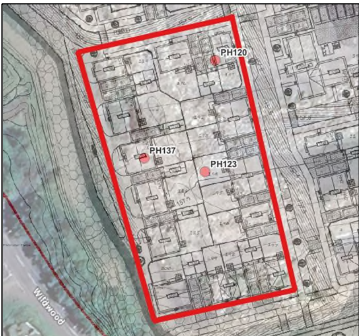
Figure 2.3 Approximate Location of Integral Geotechnique Boreholes within Study Area (NTS)
