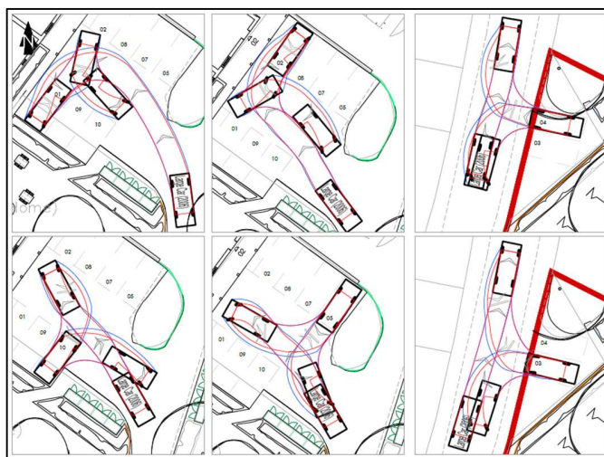
FIGURE 4.8: SWEEP PATH ASSESSMENT OF CAR PARKING SPACES
