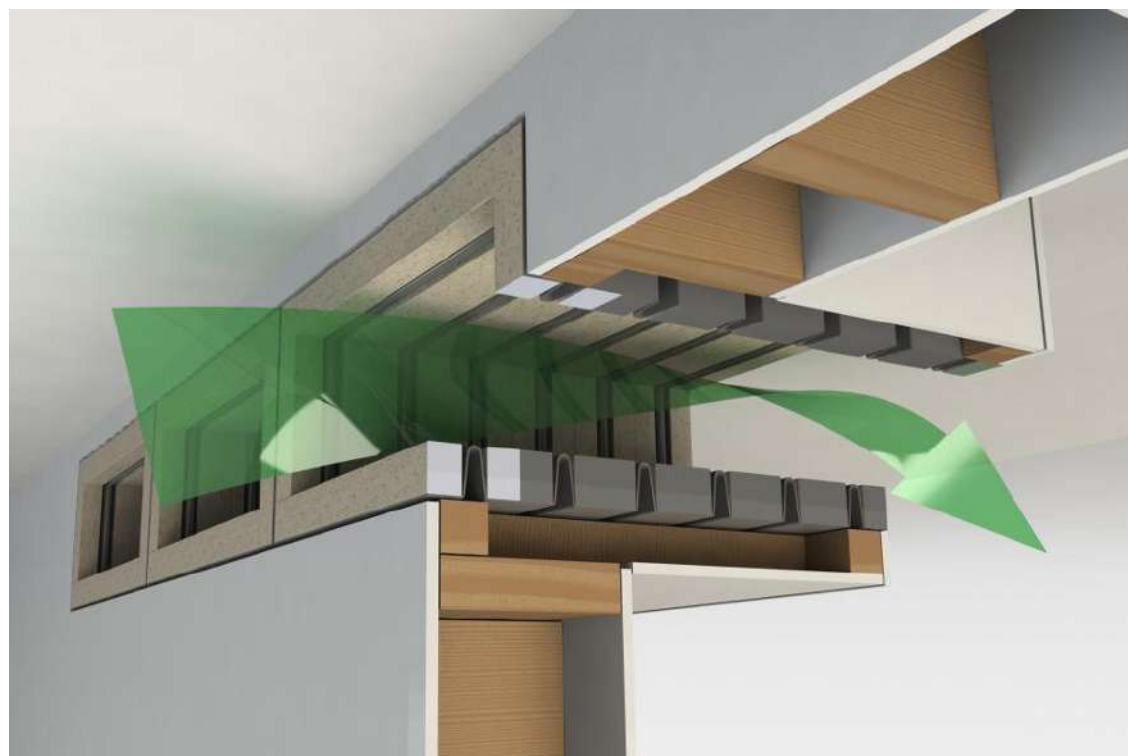
Figure 4.4 Passivent SoundScoop – Cross vent unit for summer and winter time ventilation
