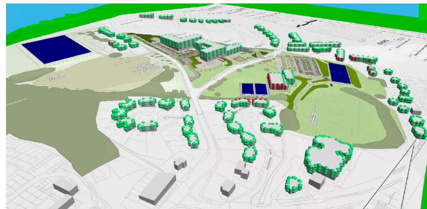
Figure 6.1: CadnaA noise mapping
