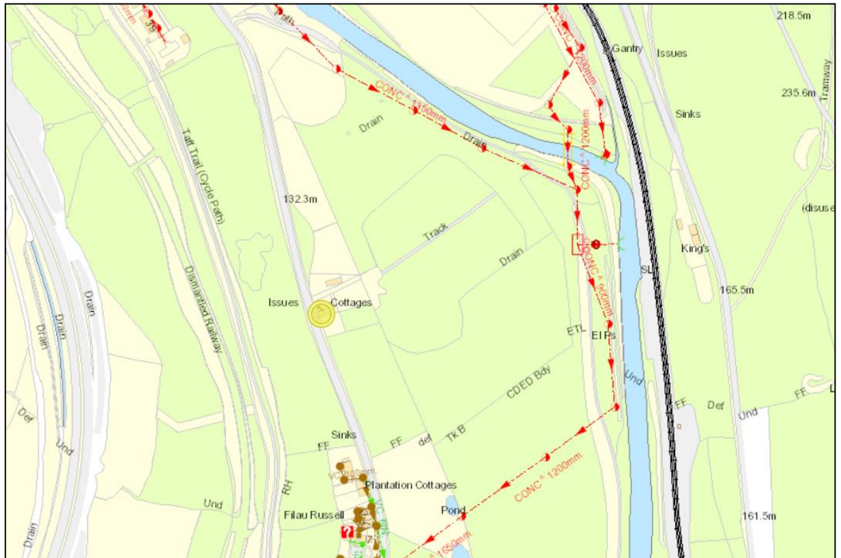
Figure 11.1 – DCWW Public Sewer Records
