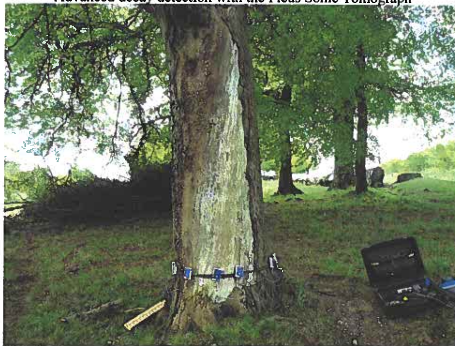
Advanced decay detection with the Picus Sonic Tomograph
