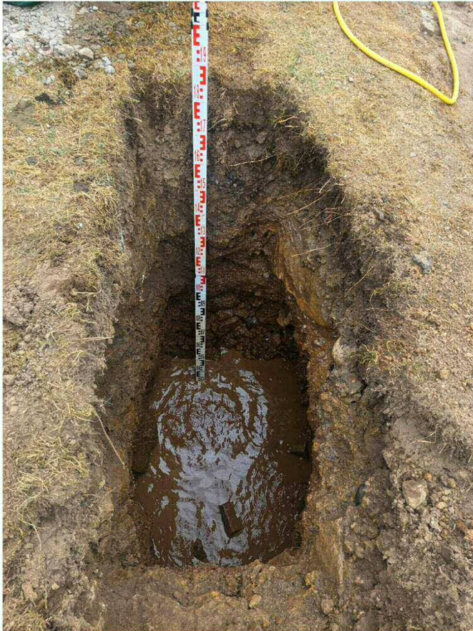
Figure 7 - Test pit 2 during filling
