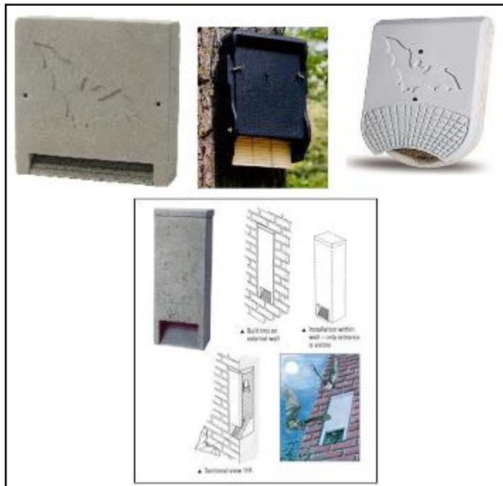
Middle: The Beaumaris bat box is made entirely from Woodstone, a robust material comprising concrete and wood fibres. This means that, not only does the box have excellent insulating properties maintaining a more consistent temperature throughout the year, it also provides excellent protection from predators. The Beaumaris box has a single narrow cavity which makes it suitable for crevice roosting bats. The interior of the box has a rough surface for bats to cling to and the front of the box features a subtle but attractive imprint of a bat in flight. It is suitable for attaching to external walls and available in two sizes: Midi and Maxi.
