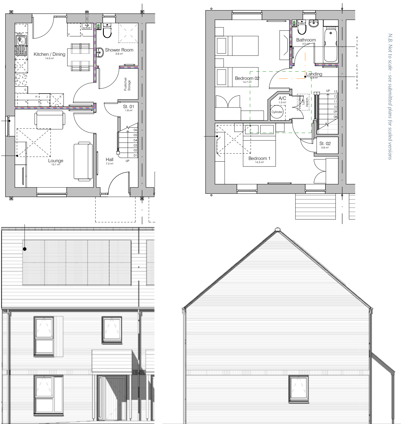
Figure 39 - House Type B Floor Plans and Elevations
