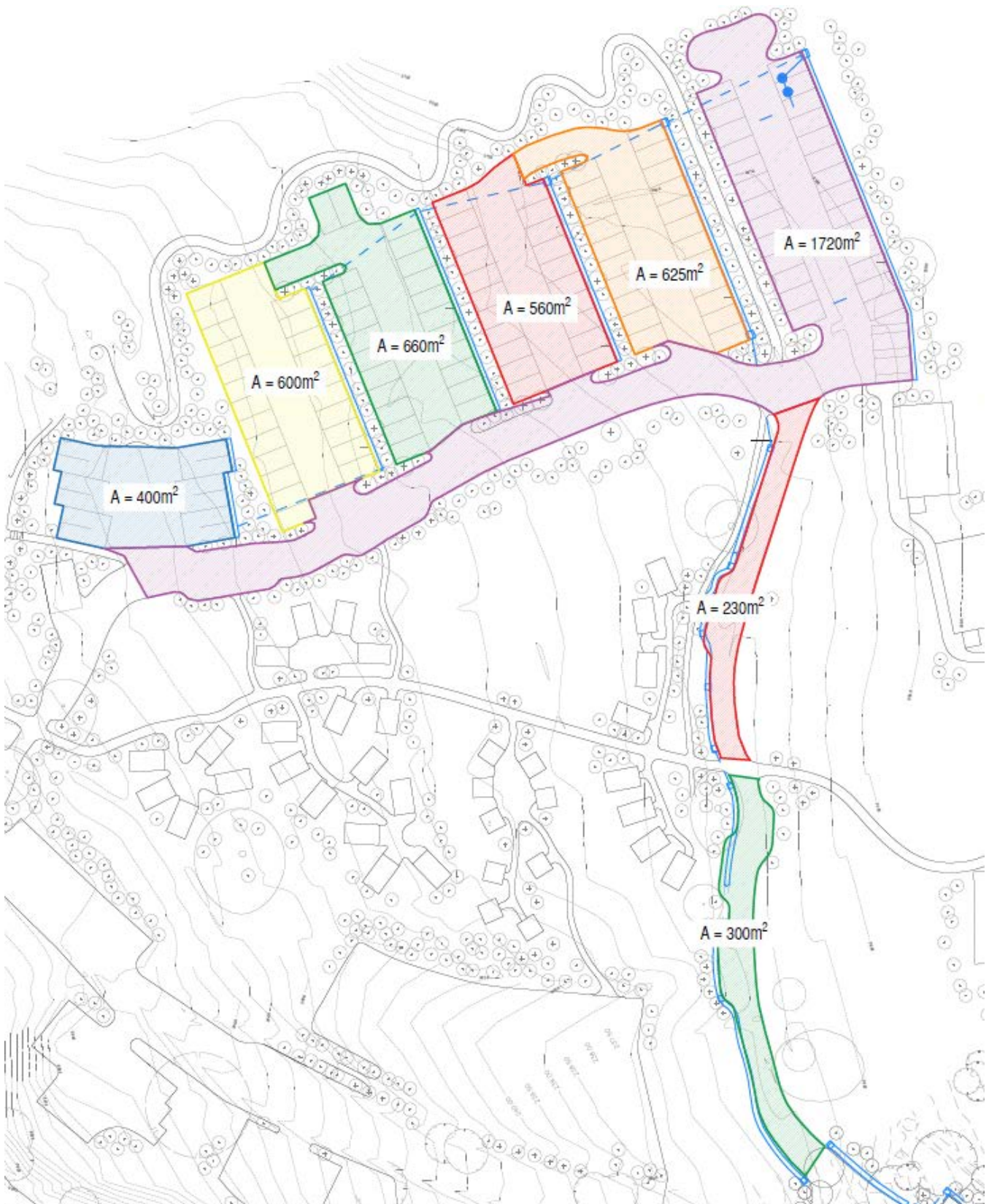
Figure 1. Drainage Areas Considered in the Network 1 Simulation
