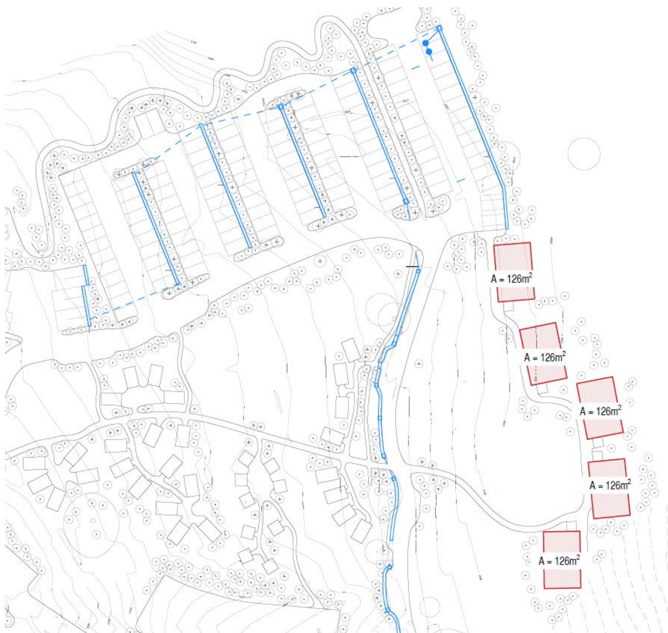
Figure 3. Drainage Areas Considered in the Network 2 Simulation
